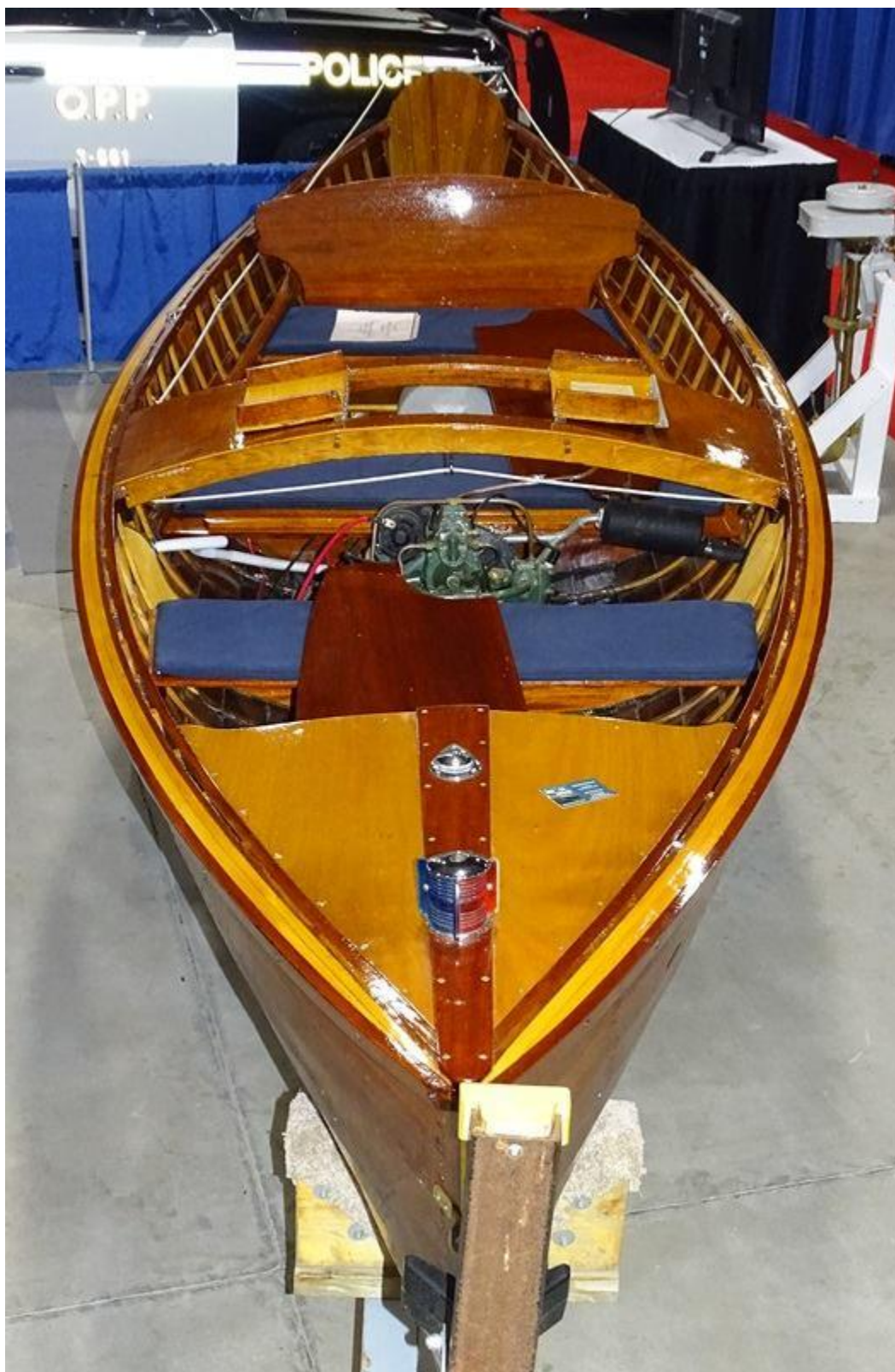
The final iteration of the Dispro, built by Greavette up to 1957 with Coventry Victor 6 hp engine Manotick Classic Boat Club photo
