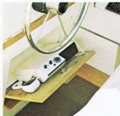
Radio storage box
