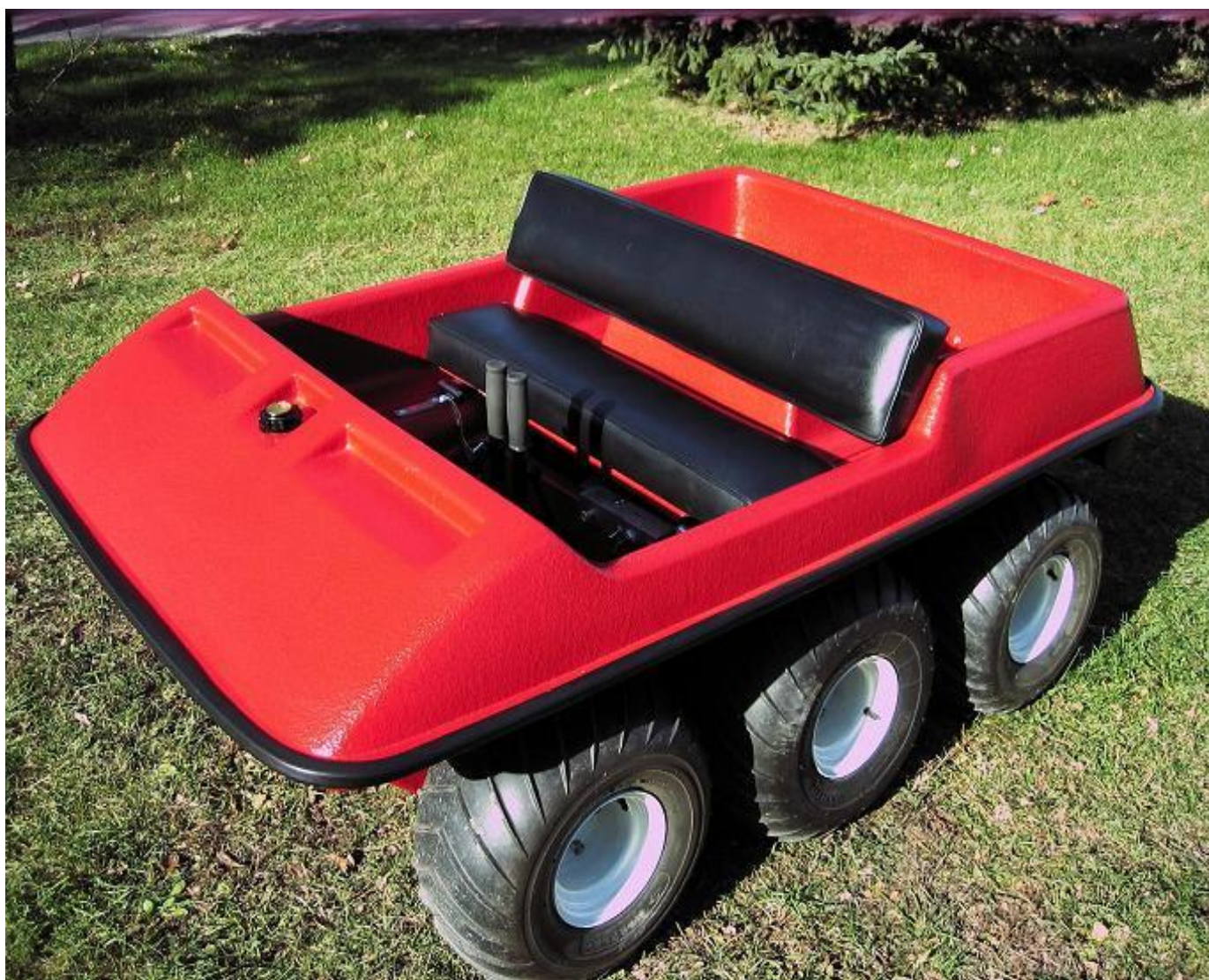
Bazooo, with two steering control handles at center of console Photo Owen1983
