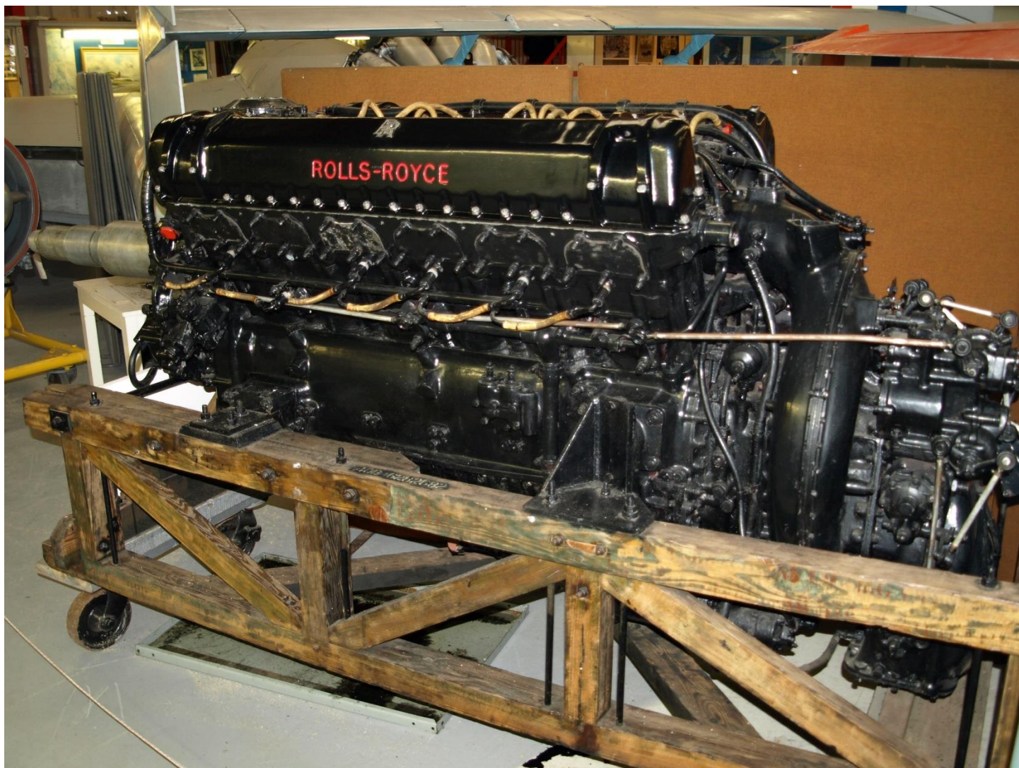
The Rolls-Royce Griffon, powering Miss Supertest's II and III Photo Nimbus 227
