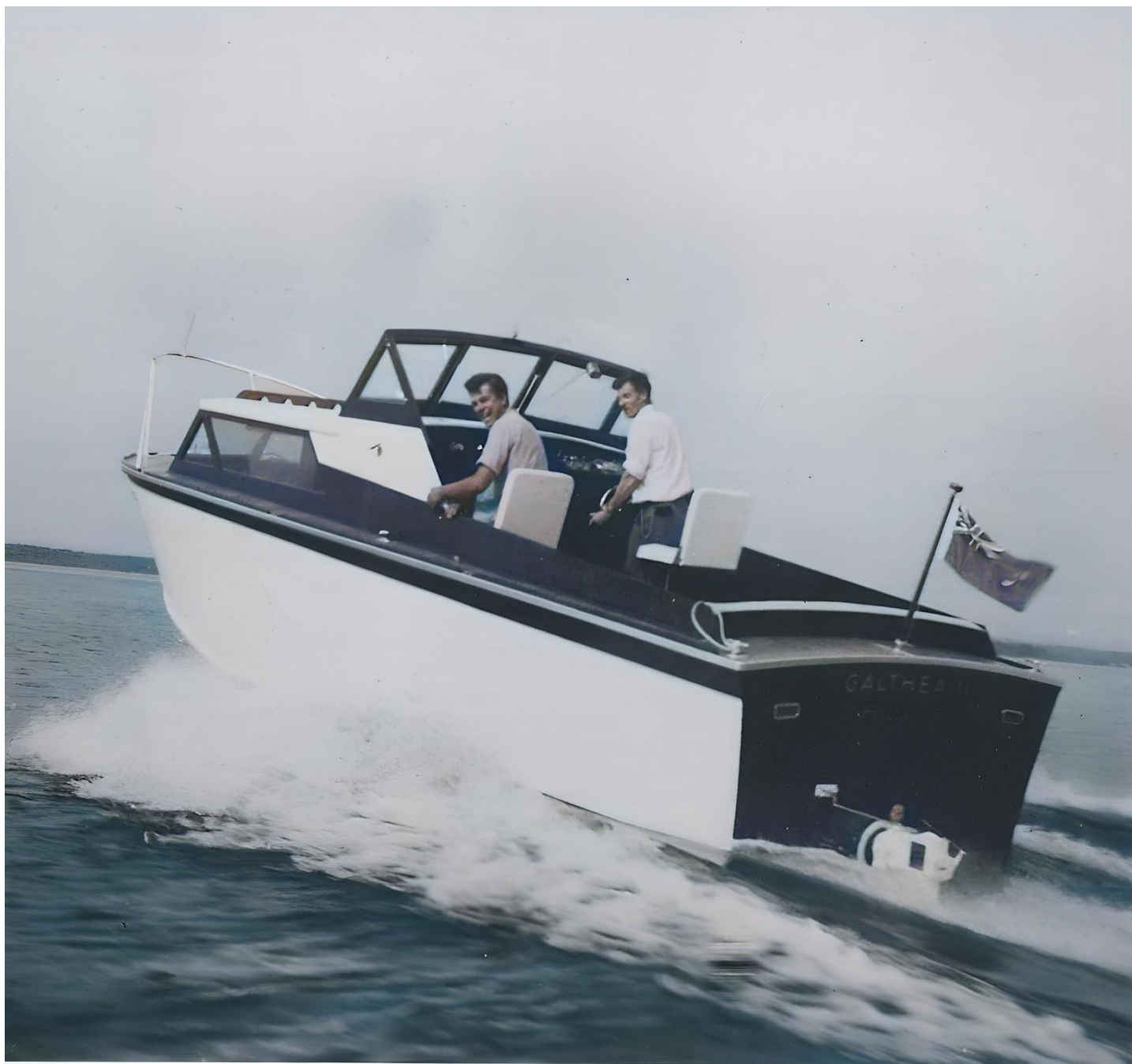
The top of the line of Ayling and Ramage, a 25-foot cruiser with a 100 hp Ford Interceptor engine. Peter Ayling is on the right, at the controls.
