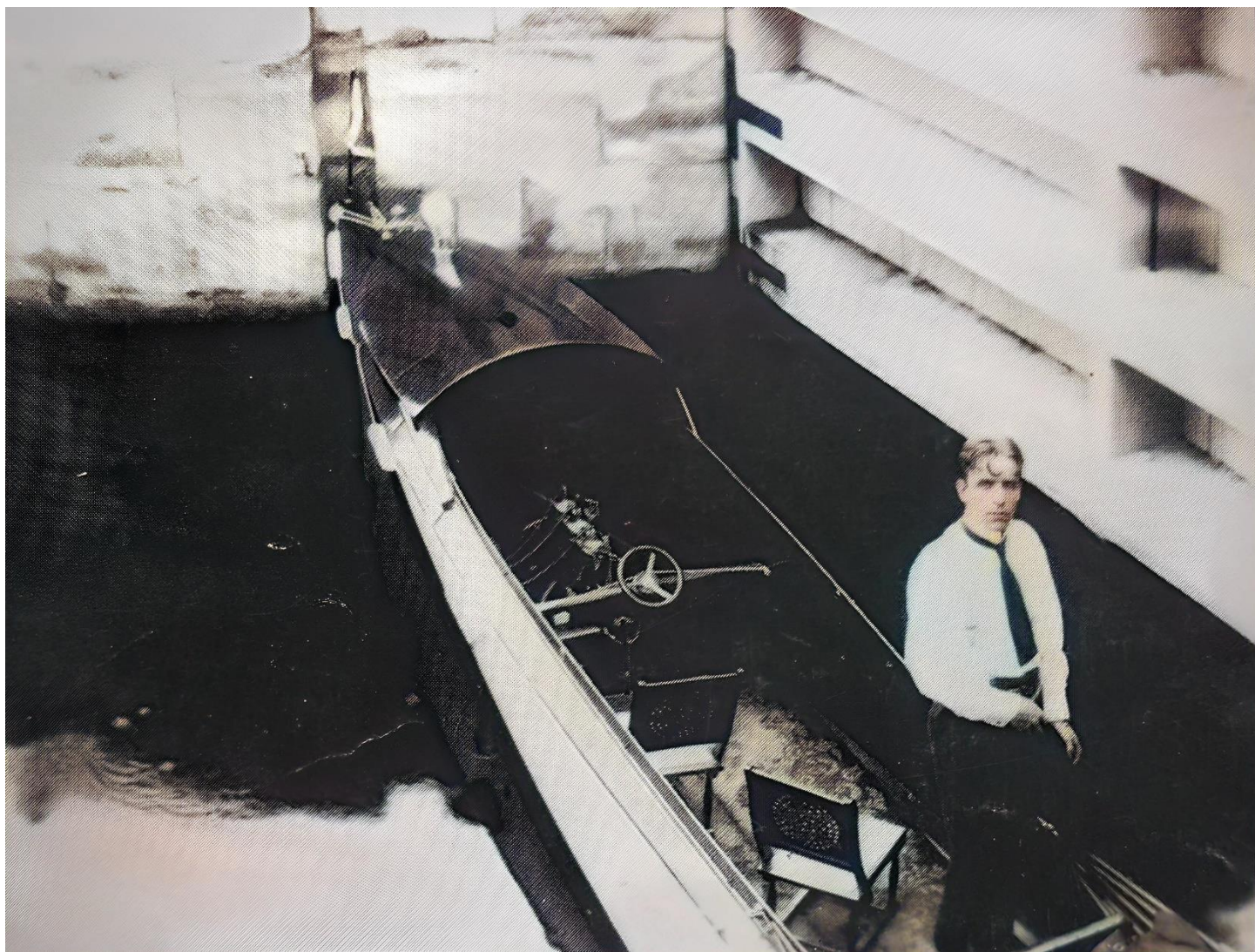
“Stuffing Box Bill”, early motorboat enthusiast, in Chaffey’s Locks. This is the private-branded St. Lawrence skiff model 2548, powered with a three-cylinder St Lawrence engine, 12 hp. Alfred Pennock
