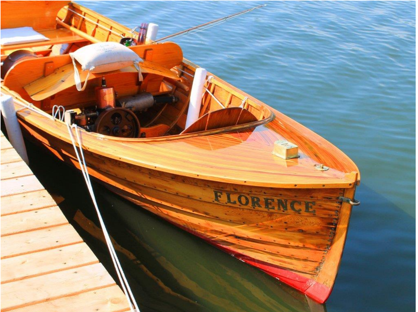
First production run Dispro, showing engine placement Manotick Classic Boat Club photo
