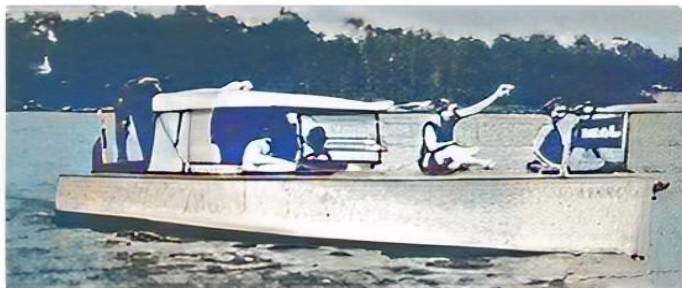
Gidleyford side view shows the windscreen, khaki colour top and "one man" top irons. All of these were "off the shelf" Model T Ford parts.
