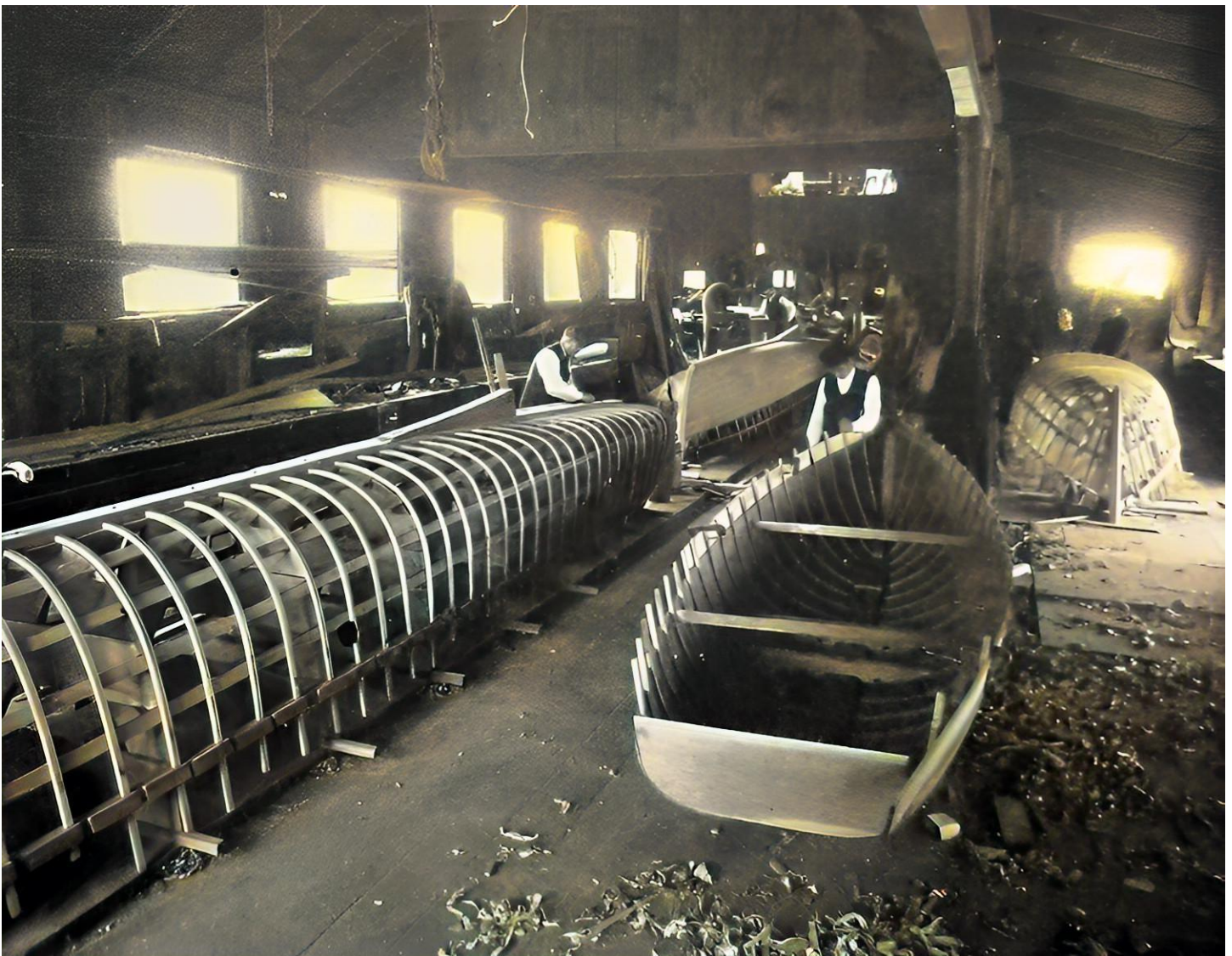
Inside the Bastien works, a long deck launch in progress at right, or at least the mould for one. The building is clearly at the Bastien works; it was also used for Robertson Bros. ads.
